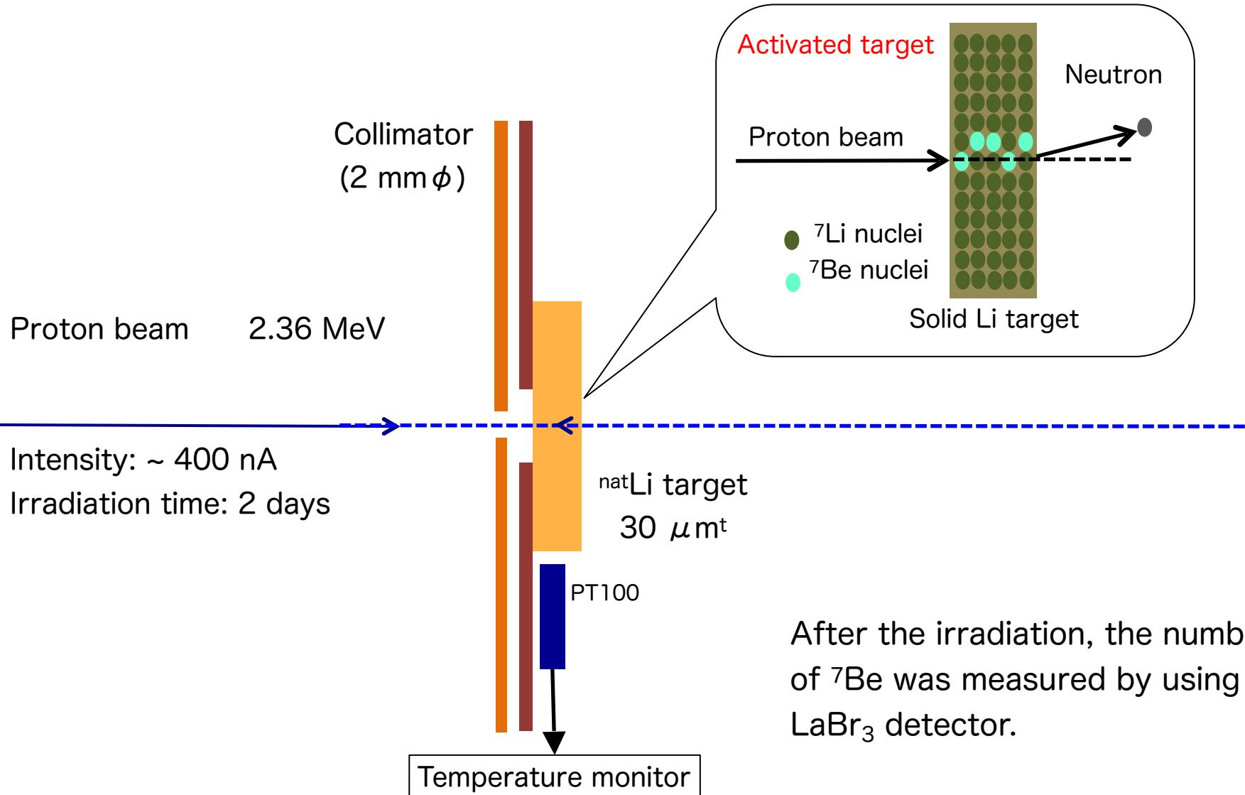
After the irradiation, the number of  ${}^7\text{Be}$  was measured by using a  $\text{LaBr}_3$  detector.
