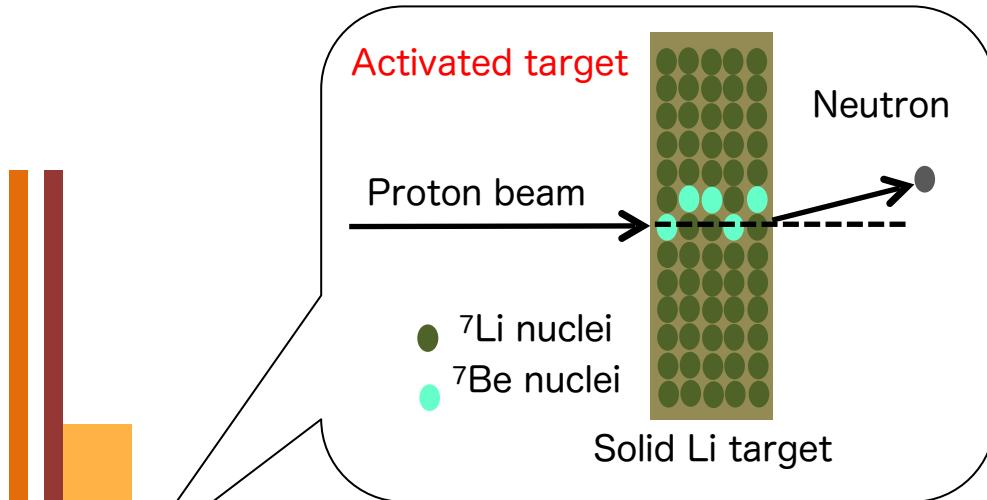
After the irradiation, the number of  $^7\text{Be}$  was measured by using a LaBr<sub>3</sub> detector.
